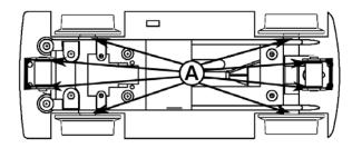
Please refer to the figure above. The wheels and roller pickups require electrical flow, therefore we recommend using Bachmann E-Z Lube® #99981 Conductive Contact Lube on all points **Marked A.**
